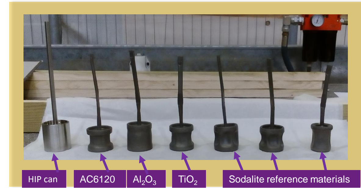
Small-scale iodine containing HIP wasteforms
