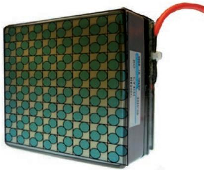
**Figure 2: MAPMT detector – with the fibre connection scheme overlaid**
