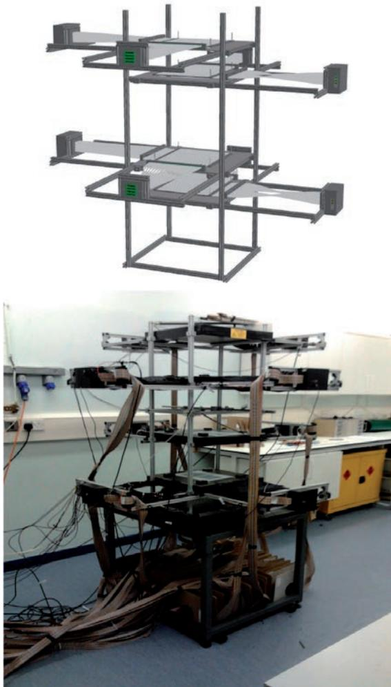
**Figure3: Top: CAD Model of the prototype imaging system, Above: Prototype Imaging system at the University of Glasgow**
